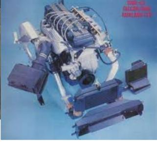
Advanced Induction Technology ("AIT") One of the premium offerings for the EA Series wa the offering of intercooled turbo kits sold through many Ford dealers. The kit used a front mount intercooler fed by extra air vents in the bumper, turbocharger, extra injectors and was signified by a build plate and instrumentation markings.
